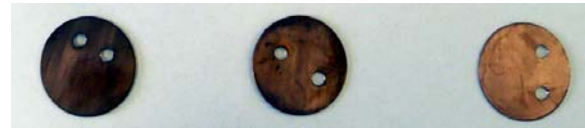
Image: Reduction In 24-Hour Corrosion Of Copper Coupons Observed During The OdorKlenz Air Stabilization Process (Before stabilization, 5 days into mitigation, and 10 days into mitigation)
