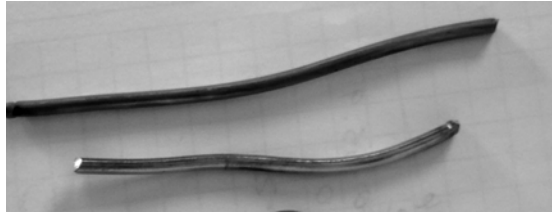
Image: There Was Substantial Corrosion Of Copper Wire In A 24-Hour Period Before OdorKlenz Air Treatment Cartridge Installation (Day 1 of Experiment | Grey-Scale Picture)
